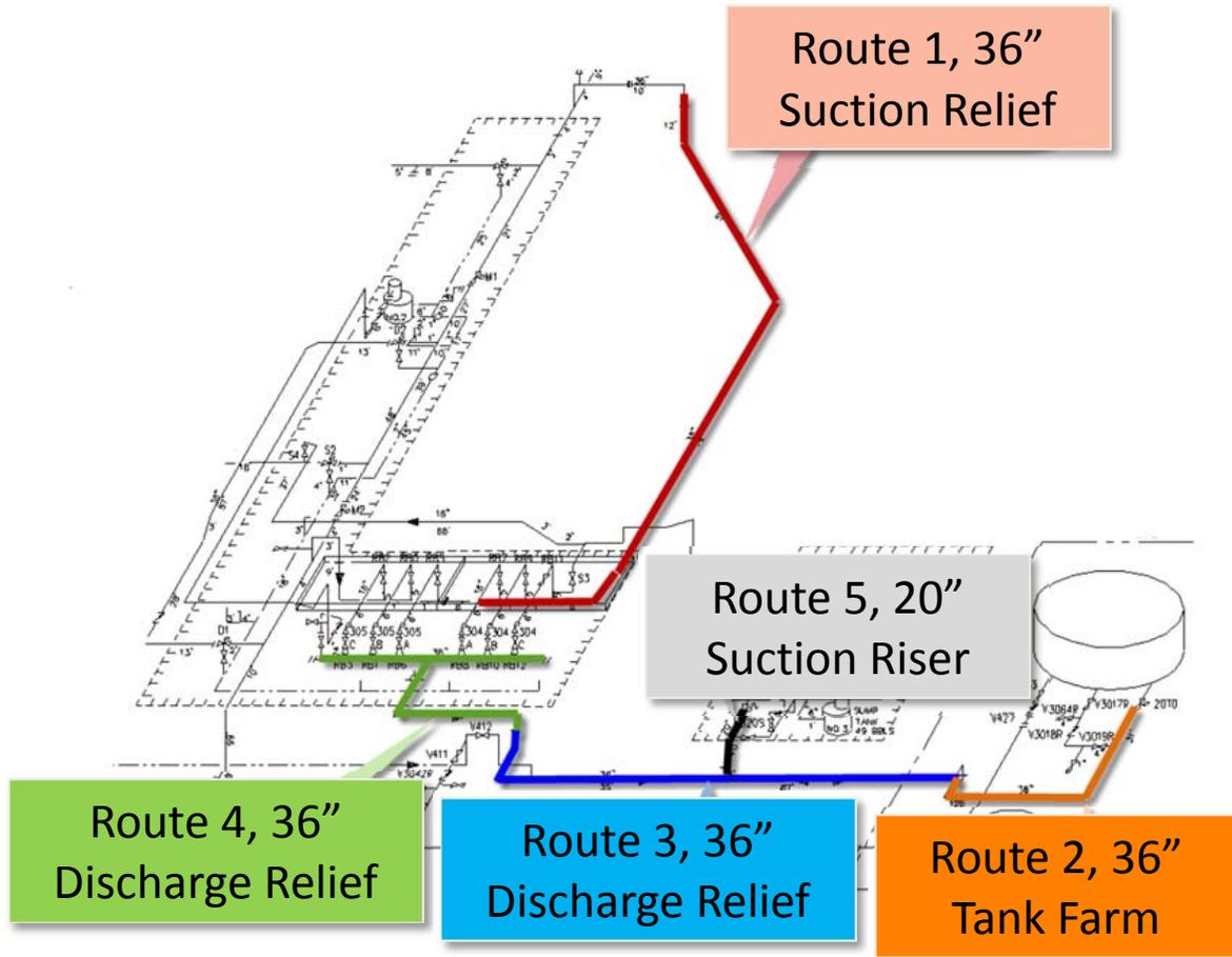
**Figure 3: Diagram of Pump Station 03 Inspection Routes**
