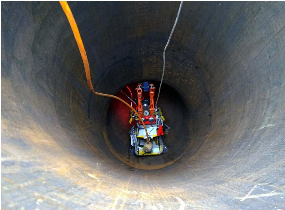
**Figure 1: Robotic ILI Crawler Vertically Entering PS03 Inspection Area**
