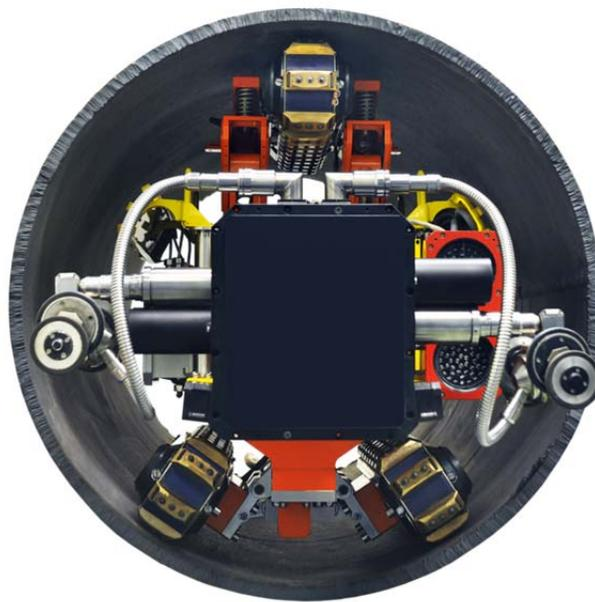
**Figure 2: Robotic ILI Crawler with Three Tracks Engaged Into the Pipe ID**
