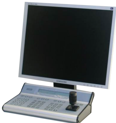
Camera control station
